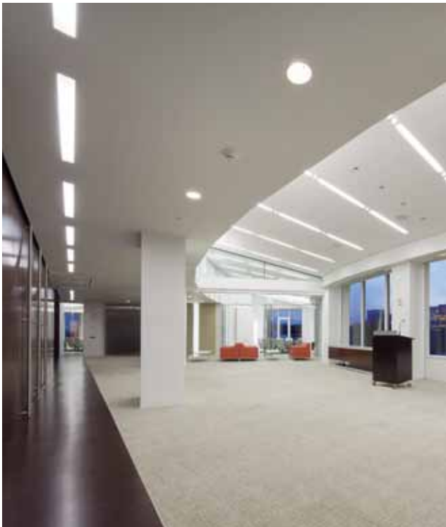
Central corridors, or “boulevards,” run the length of the building. MR16 accents and fluorescent T5s are arranged in “dots and dashes” to complement the linearity of the boulevards and highlight materials and finishes, such as the dark wood walls and white Terrazzo floors.
