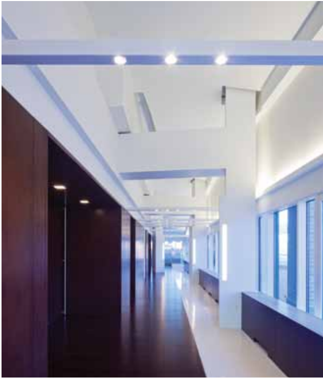
Central corridors, or “boulevards,” run the length of the building. MR16 accents and fluorescent T5s are arranged in “dots and dashes” to complement the linearity of the boulevards and highlight materials and finishes, such as the dark wood walls and white Terrazzo floors.
